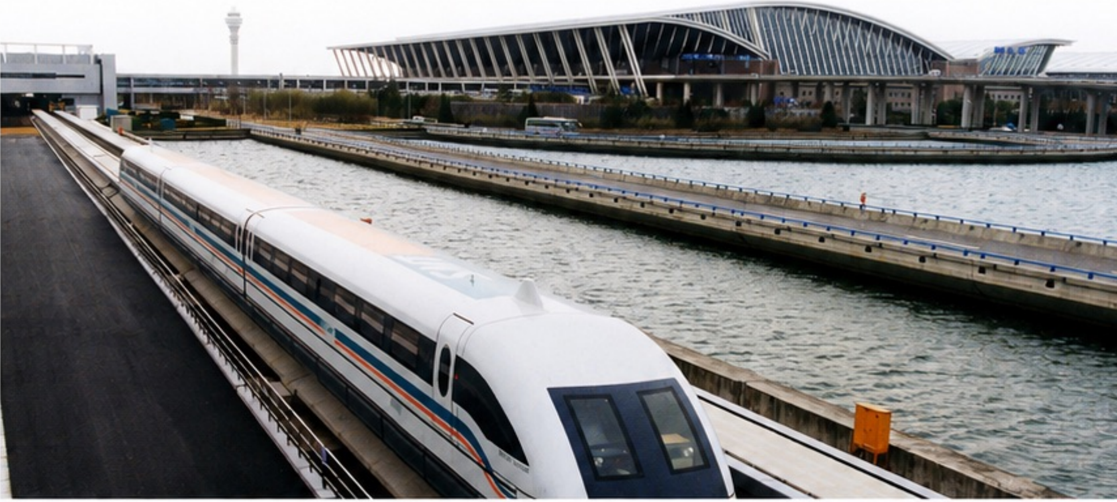
Engineers get the train to float above the tracks using electromagnetic suspension. SPECIAL ARRANGEMENT
