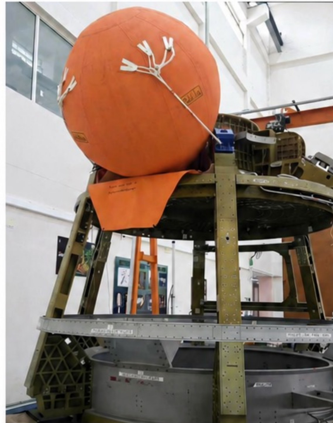
Step-by-step: (Clockwise from left) The crew module uprighting system, the service module connect-disconnect system, and the apex cover that underwent testing. ISRO
